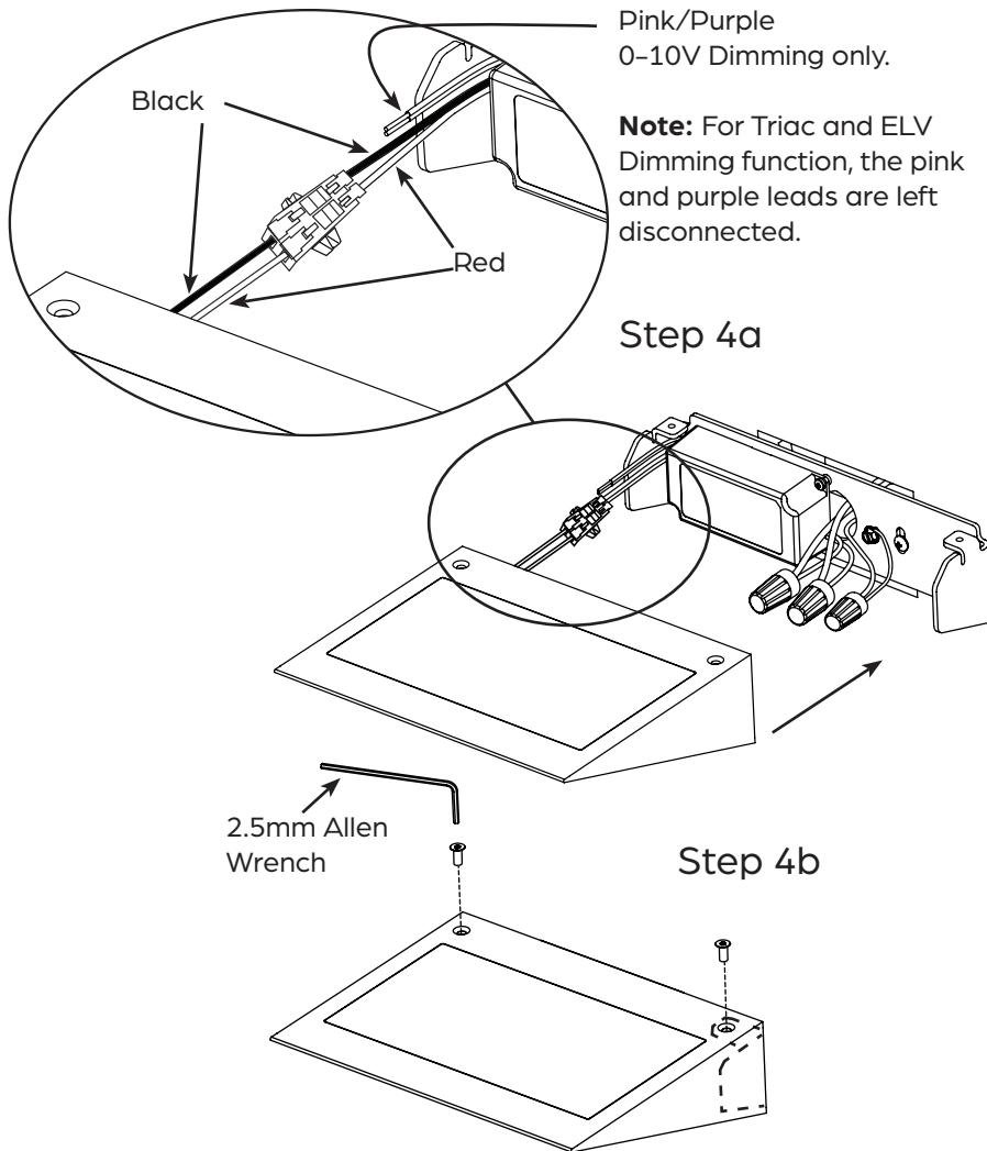
Step 4: Installation – Re-attach light unit to bracket and driver
