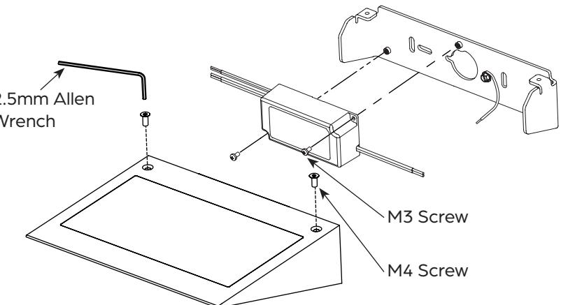
Step 1: Disassembly – Remove the bracket from the light unit.
